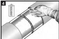
Clean exposed steel and adjacent pipe coating with a solvent cleanser that will not leave an oil residue (ie. ethanol, MEK, etc.) to remove the presence of oil, grease, and other contaminants.
