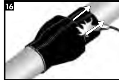
If the closure lifts while shrinking, secure it with a gloved hand. Continue heating from the bell of the tyton joint to the other end (spigot) until recovery is complete.
