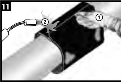
1. Clean the overlap area of the sleeve where the closure is to be applied.
