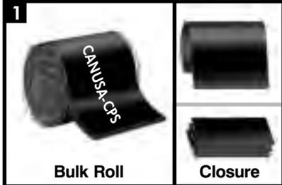
High Shrink WLOX is typically shipped in bulk rolls. Closures are shipped either in bulk rolls or pre-cut. The adhesive is protected from contamination by an inner liner. High Shrink sleeves are used with tyton, flange, coupling, and casing joint applications.
