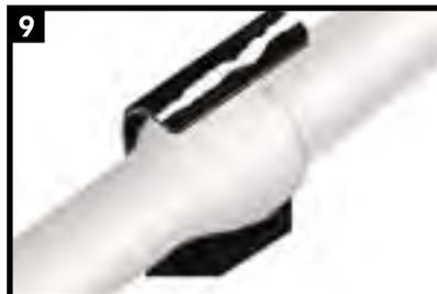
Centre the sleeve over the joint so that the sleeve overlaps between the 10 and 2 o'clock positions. Press the underlap firmly into place and remove the remaining release liner.
