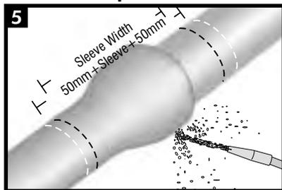
Ensure that the pipe is dry before cleaning. Prepare the steel joint area to a minimum of S12/SP2. Lightly abrade the pipe coating adjacent to the weld area to a distance of 50mm (2") beyond each end of the sleeve width.
