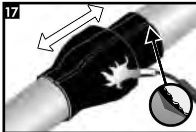
In a similar manner, heat and shrink the remaining side. Shrinking has been completed when the adhesive begins to ooze at the sleeve edges all around the circumference.
