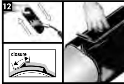
Warm the adhesive side of the closure until it becomes shiny. Centre the closure over the overlap. Using a gloved hand press the closure firmly down onto the overlapping sleeve.
