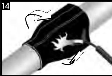
Using broad strokes, begin shrinking the WLOX sleeve around the entire circumference of the larger end (bell) of the tyton joint. Continue heating from the centre of the sleeve until sleeve recovery is completed around the bell of the tyton joint.
