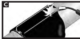
Wrap the sleeve loosely around the pipe, ensuring the appropriate overlap. Gently heat the backing of the underlap and the adhesive side of the overlap.
