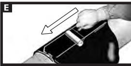
Wrap the sleeve loosely around the pipe, ensuring the appropriate overlap. Gently heat the backing of the underlap and the adhesive side of the overlap.
