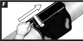
Gently heat the closure and pat it down with a gloved hand. Repeating this procedure, move from one side to the other. Smooth any wrinkles by gently working them outward from the centre of the closure with a roller.
