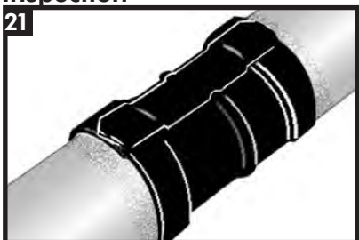
Visually inspect the installed sleeve for the following: • Sleeve is in full contact with the steel joint. • Adhesive flows beyond both sleeve edges. • No cracks or holes in sleeve backing.
