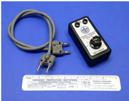
Enter the *Ref-Check*, which is designed to verify the serviceability (health) of a permanent or portable reference electrode. While we can't change the circuit resistance of earth or water, we can impose various levels of resistance in parallel with the DMM. By changing the circuit resistance, we can then determine whether or not the reference electrode is providing accurate readings.
