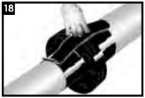
Using a gloved hand, apply the closure over the flange clips as additional protection.
