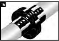
Gently push down the sleeve so it conforms to the flange profile.
