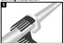
Wrap the finger skirting around one half of the flange. The fingers should point towards the flange bolts.
