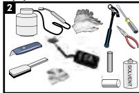
Propane tank, hose, torch & regulator. Appropriate tools for surface abrasion. Knife, roller, rags & approved solvent cleanser. Temperature measuring device. Hammer, small flat-head screw driver, needle-nose pliers. Standard safety equipment; gloves, goggles, hard hat, etc.
