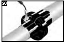
Apply an even final heating to the entire closure seal.
