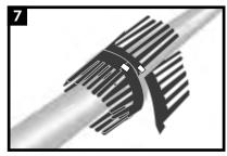
Centre the protective skirting over the flange. Using the tape provide, attach the skirting to the flange. Begin wrapping the protective skirting around flange tightly.
