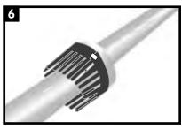
Finish wrapping the skirting around the flange. Use a piece of tape to secure the skirting in place.
