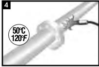
Using an appropriate heating device, pre-heat the pipeline to 50°C (120°F) (warm to the touch) and heat the flange to remove moisture.
