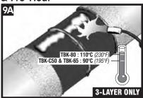
Pre-heat the epoxy and abraded coating to the required temperature with the appropriate propane torch. This will substantially cure the epoxy and ensure proper flow and bonding of the sleeve adhesive. Ensure that the epoxy primer is dry to the touch prior to sleeve installation. If a film develops on the mainline coating because of preheat, use a surface abrasion tool to remove it.
