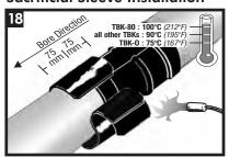
Ensure that the front 100mm (4") of the first sleeve and 100mm (4") onto the coating is at the required temperature. Completely remove any release liners from the 150mm (6") sacrificial sleeve. Wrap the 150mm (6") sacrificial sleeve so that half of the sleeve overlaps the first sleeve and half of the sleeve extends onto the coating. Position the closure on the opposite side of the pipe relative to the first sleeve closure. Recover the sleeve as in steps 10 through 17.
