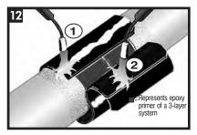
Wrap the sleeve loosely around the pipe, ensuring the appropriate overlap. Gently heat the backing of the underlap (1) and the adhesive side of the overlap (2). For TBK-80, heat the adhesive side of the closure until it becomes shiny.
