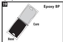
Follow the Preparation, Mixing and Application instructions provided with the supplied Canusa Epoxy Pack. For bulk quantities: mix the primer cure with the primer base (4 parts base to 1 part cure ne). Stir for a minimum of 30 seconds to assure uniform
