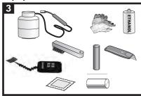
Canusa torch, propane tank, hose & regulator Temperature measuring device, roller, knife Appropriate surface abrasion device, solvent Standard safety equipment (gloves, goggles, hard hat, etc.) Wet film thickness gauge
