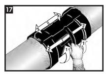
While the sleeve is still hot and soft, use a hand roller to gently roll the sleeve surface and push any trapped air up and out of the sleeve, as shown above. Continue the procedure by also firmly rolling the closure with long horizontal strokes from the weld outwards
