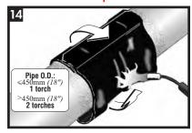
Using the appropriate sized torch, begin at the centre of the sleeve and heat circumferentially around the pipe. Use broad strokes. If utilizing two torches, operators should work on opposite sides of pipe.
