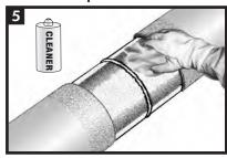
Clean exposed steel and adjacent pipe coating with a solvent cleaner to remove the presence of oil, grease, and other contaminants. Ensure that the mainline coating edges are bevelled to  $30^\circ$ .
