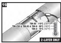
Pre-heat the cutback area and abraded coating to the required temperature with the appropriate propane torch. Ensure the correct temperature has been reached using a temperature measuring device. If a film develops on the mainline coating because of preheat, use a
