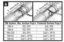
Ensure the pipe is dry before abrading. Using the chart above, abrade the pipe to the required cleanliness. Lightly abrade the line coating adjacent to the weld area to a distance 225mm (9") beyond the sleeve width on the front-end and 150mm (6") beyond the sleeve width on the back-end. Wipe clean or air blast the steel and pipe coating to remove foreign contaminants.
