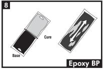
Follow the Preparation, Mixing and Application instructions provided with the supplied Canusa Epoxy Pack. For bulk quantities: mix the primer cure with the primer base (4 parts base to 1 part cure **by volume**). Stir for a minimum of 30 seconds to assure uniform mixture.
