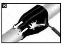
Continue shrinking from the bell of the tyton joint to the sleeve end. Sleeve recovery is complete when it conforms to the pipe.
