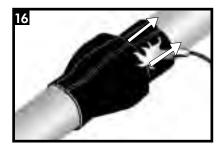
If the closure lifts while shrinking, secure it with a gloved hand. Continue heating from the bell of the tyton joint to the other end (spigot) until recovery is complete.
