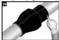
With a gloved hand, press down on the installed sleeve to ensure the backing and sleeve are soft. If there are any cool spots, the sleeve should be reworked with additional heat.
