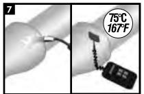
Pre-heat the joint area to a minimum of 75°C (167°F). Using a temperature measuring device, ensure that the correct temperature is reached on the steel and at least 50 mm (2") on each side of the sleeve.
