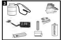
Propane tank & torch Appropriate tools for surface abrasion Knife, roller, rags & solvent cleanser Temperature measuring device Standard safety equipment; gloves, goggles, hard hat, etc.
