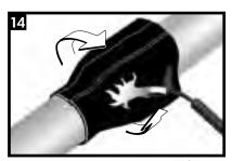
Using broad strokes, begin shrinking the WLOX sleeve around the entire circumference of the larger end (bell) of the tyton joint. Continue heating from the centre of the sleeve until sleeve recovery is completed around the bell of the tyton joint.
