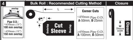
As a guideline, cut the required lengths of Sleeve material (L) and Closure material (W) from the bulk roll as follows  $\mathbf{L} = \mathbf{Coated\ Pipe\ circumference} + \mathbf{overlap\ dimension}$
