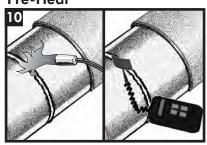
Pre-heat the joint area to the minimum required temperature (see Surface Preparation & Pre-Heat Chart). Using a temperature measuring device, ensure that the correct temperature is reached on the steel and at least 50mm (2") on each side of the sleeve.
