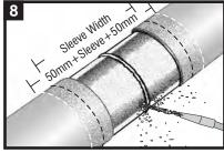
Ensure that the pipe is dry before cleaning. Prepare the steel joint area using the Surface Preparation and Pre-Heat Chart as a guideline. Lightly abrade the pipe coating adjacent to the cutback area to a distance of 50mm (2") beyond each end of the sleeve width.
