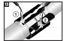
Wrap the sleeve loosely around the pipe, ensuring the appropriate overlap. Gently heat the backing of the underlap and the adhesive side of the overlap. Press the overlap into place.
