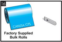
Measure the circumference of the of pipe and cut two (2) lengths of Wrapid Bond at a length equal plus 75mm (3").
