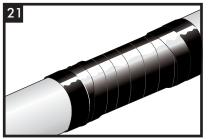
Apply a circumferential wrap around the pipe at a  $90^{\circ}$  angle overlapping the factory coating by 50% of the tape width.
