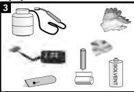
Propane tank, hose, torch & regulator Appropriate tools for surface abrasion Knife, roller, rags & approved solvent cleanser Digital thermometer with suitable probe Standard safety equipment; gloves, goggles, hard hat, etc.
