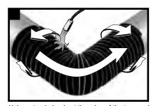
Using a torch, begin at the edge of the tape and heat circumferentially around the joint, working back to the other edge.
