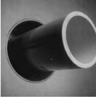
1. Center the pipe, cable or conduit in wall opening or casing. Make sure the pipe will be adequately supported on both ends. Link-Seal® modular seals are not intended to support the weight of the pipe.
