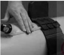
6. Insert all Slide-Locks as far as possible by hand. Complete tightening by tapping each Slide-Lock with a hammer, while holding the Slide-Lock against the pipe.
