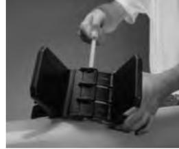
3. Locate the directional arrows on the segment and insert Slide-Lock until the tip exits the end of the segment.
