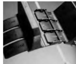
C) Take a Slide-Lock and insert the opposite direction of the arrows. Push until you can grab the broken piece and remove.
