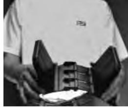
2. Take the segments and align the buckles. Insert the buckles 1/4 of the way into the slots. This will vary after your first installation.
