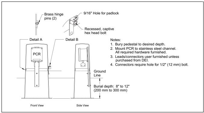
Typical Installation for AC Voltage Mitigation
