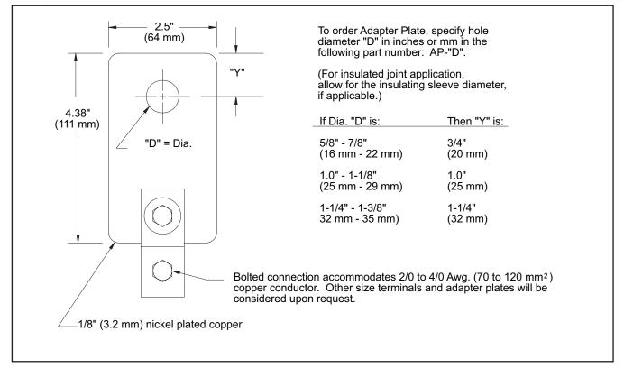
Web Tab Mounting of a PCR for Over-Voltage Protection of an Insulated Joint
