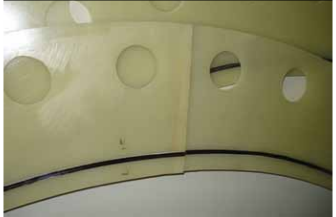
The gasket for a water project failed the initial hydrotest.
