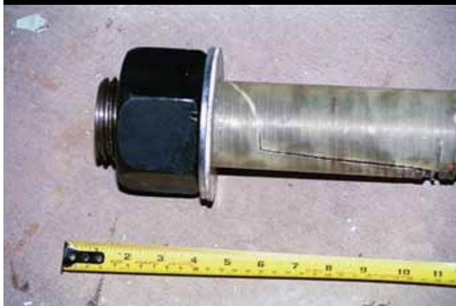
Bolt sleeve failure from shear stresses.
