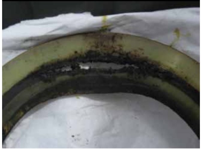
A gasket from a treated water dump.
