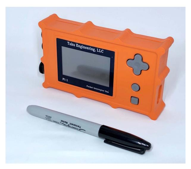
The Taku Engineering Pocket Interrupter One (Pi-1) is a hand held, light weight three channel GPS time synchronized cathodic protection (CP) current interrupter. By its self, the Pi-1 is capable of interrupting two CP current sources of up to 1 amp and 20 volts each. All three interruption channels provide standard On/Off cycles from 1 second to 30 seconds long. With a Mobiltex external high current relay connected to it, a Pi-1 can interrupt up to 100 amps and 100 volts.
