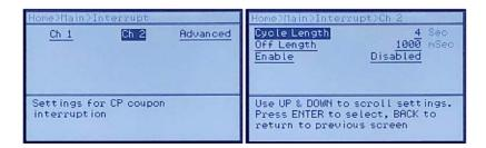
Channel Two (CH2) is a special testing/coupon interruption channel. The maximum current handling of this channel is 1 amp, and the maximum voltage is 20 volts. The connections for CH2 are provided via the Multi-Port connector located on the bottom left hand side, end panel of the interrupter. These connections are broken out to banana jack leads in the charge adapter cable. CH2 is also <u>not</u> polarity sensitive. When CH 2 is enabled, the impressed current feature of CH 1 is disabled.
