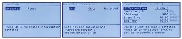
Channel one (CH1) is the main interruption channel and is used for everyday instant off survey interruption. This channel can be used for either galvanic or rectifier interruption. When set to "GALVANIC", the internal solid state relay is engaged. The maximum current handling of the CH1 internal relay is 1 amp, and the maximum voltage is 20 volts. The banana jack connections for this channel are on the left hand side of the unit, and are **not** polarity sensitive.
