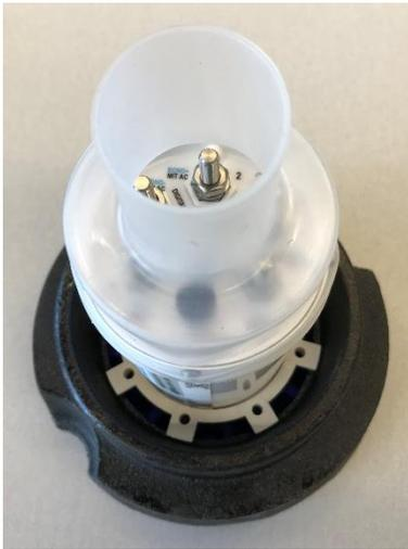
**Figure 4 RMU1-SUB ready for screws**
