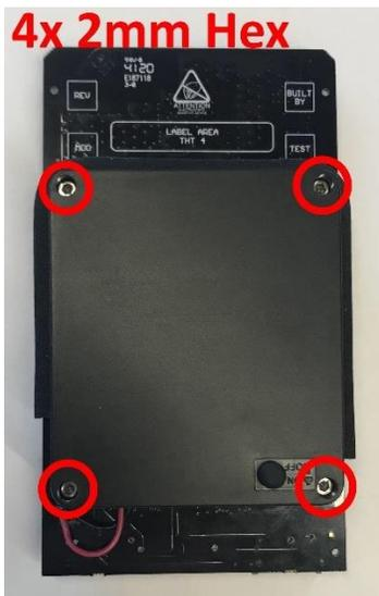
**Figure 34 Remove the 4 screws using a 2mm Hex driver**
