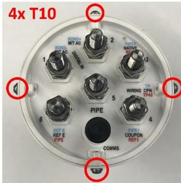
Figure 32 Remove the 4 T10 Torx screws around the sides
