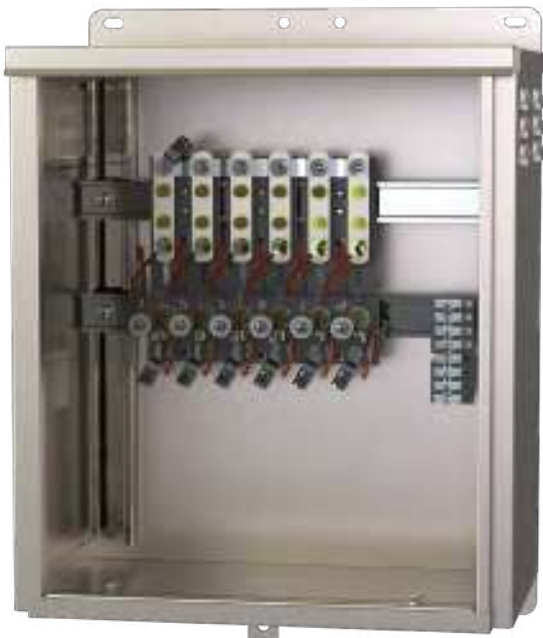
Figure 1: A typical UltraBox configuration using an 18"Hx16"Wx10"D stainless steel enclosure with dual horizontal DIN rails, six shunt and resistor modules and an isolated terminal module.
