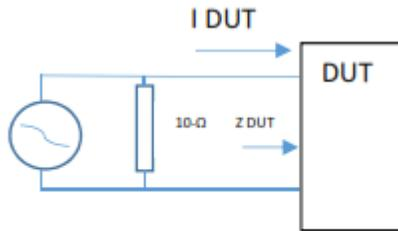
**Figure H-5: Equivalent Circuit – Source Currents to DUT.**
