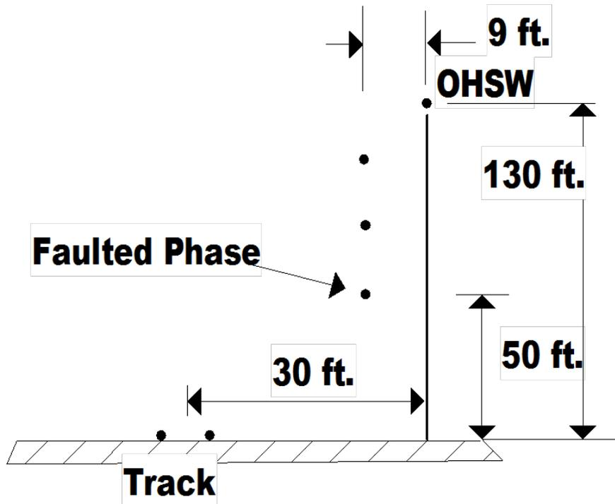
**Figure L-2. Cross-Section Geometry in Exposure**
