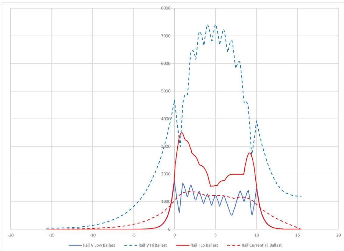
**Figure L-5: Composite Calculated Maximum Rail Voltage and Current versus Fault Location Along Exposure for Low & High Values of Track Ballast Resistivity**
