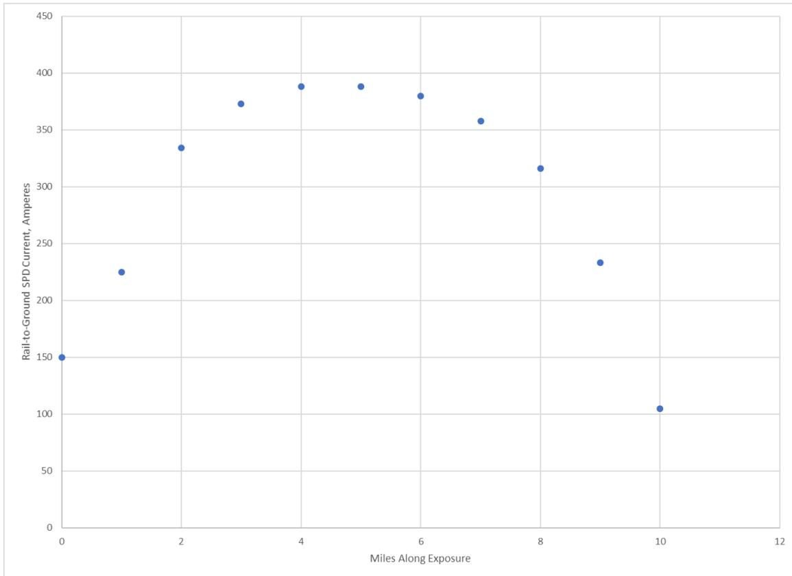
**Figure L-8: Calculated Maximum Fault-Induced Current through Rail-to-Ground HEFPDs at non-IJ Locations**
