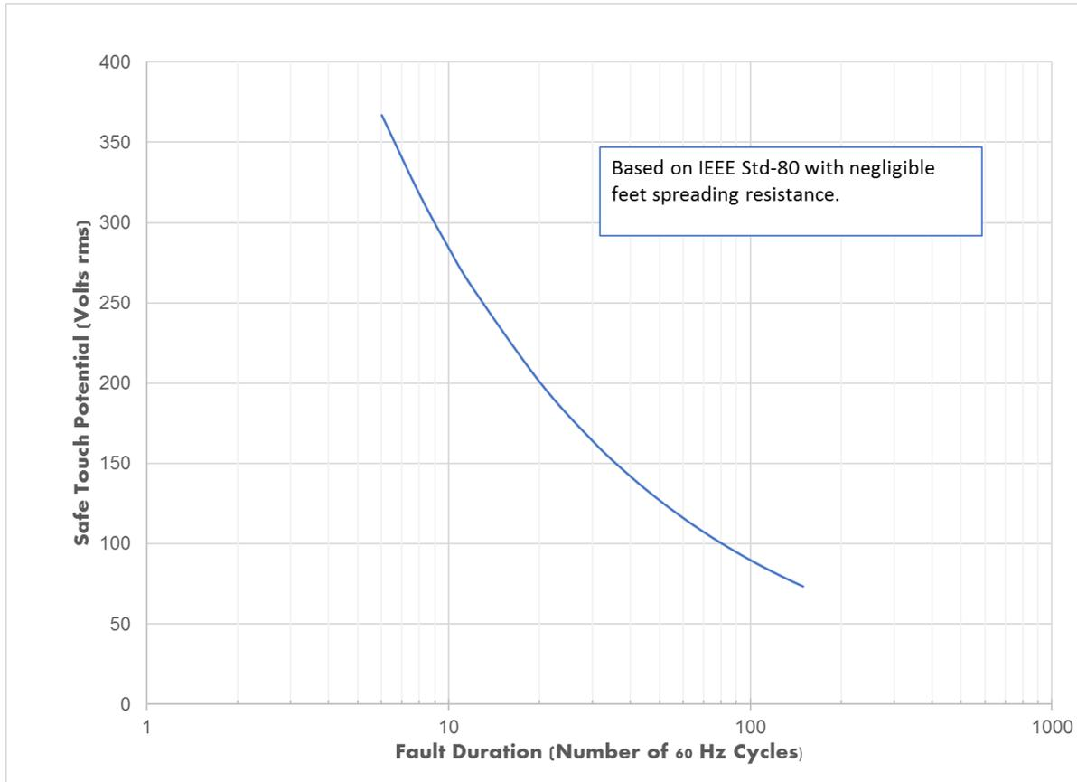
**Figure E-1: Safe Touch Potential vs Fault Duration Using Eq. 2.**
