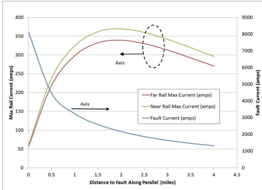
**Figure F-5: Fault Current and Induced Rail Current for Various Fault Locations for a 12 kV Distribution Line With a Neutral Wire**
