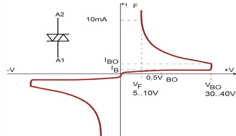
**Figure B-1: Voltage Current Characteristic Representative of a Crowbar Device.**
