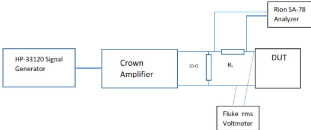
**Figure H-1: Harmonic Test Arrangement for Lab Test**
