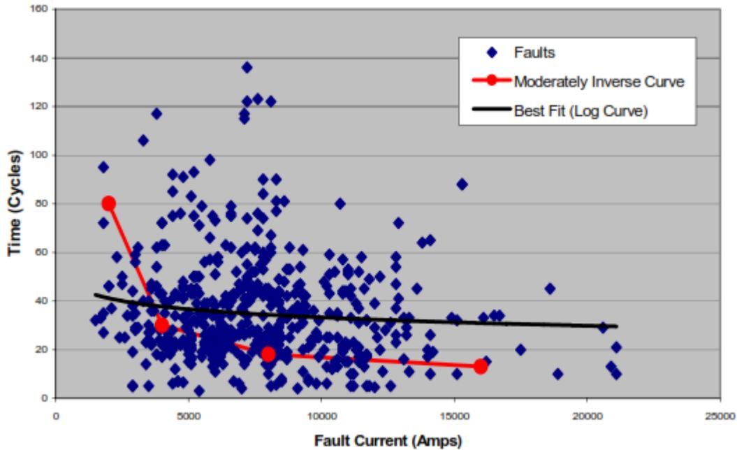
**Figure E-2: Distribution Line Fault Current Vs. Duration in 60 Hz Cycles From Reference 2.**
