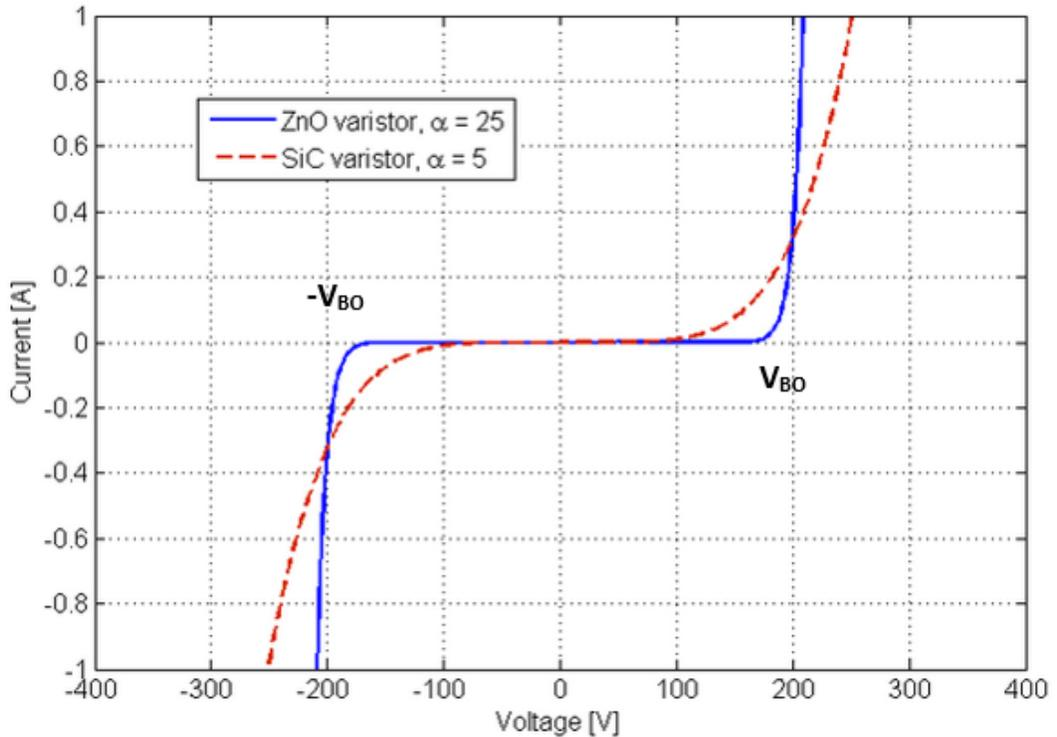
**Figure B-2: Voltage Current Characteristic of Clamping Device.**
