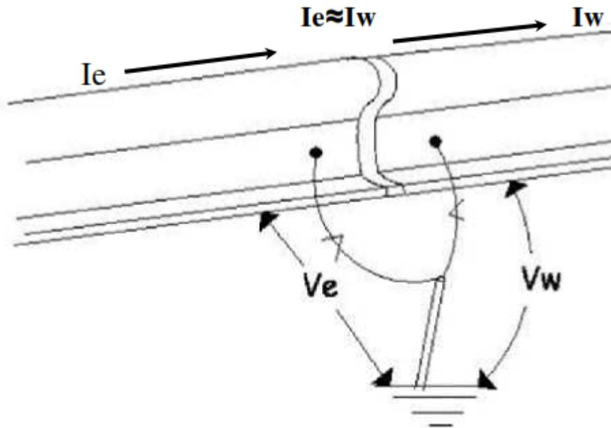
**Figure L-4: Sketch of Rail Insulated Joint with HEFPD Electrically Connected from Rail-to-Ground on Each Side of the IJ.**
