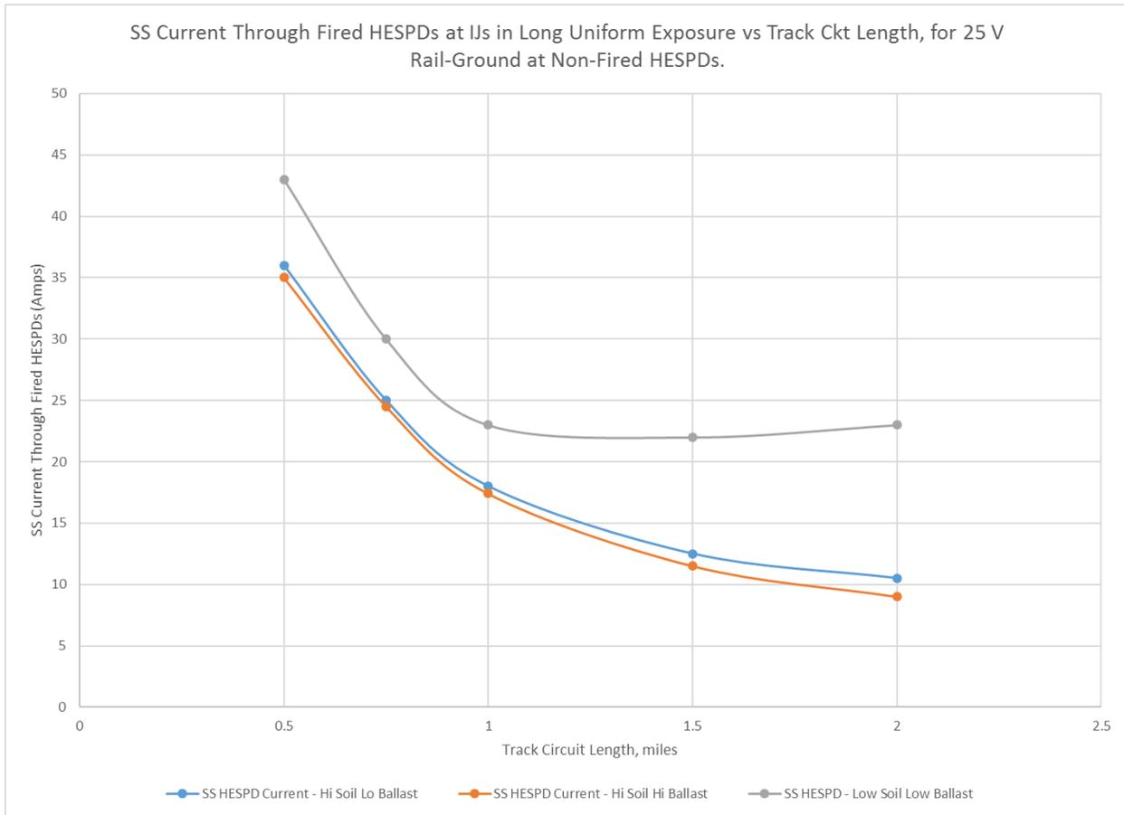
**Figure K-1: Calculated Steady-State Current Through Fired HEFPD at IJs.**
