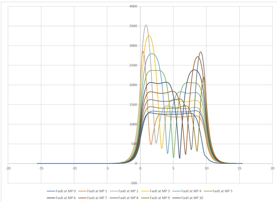
**Figure L-6. Fault-Induced Rail Current Curves for Faults at One-mile Increments Along the Parallel Exposure for Low Assumed Track Ballast Resistivity.**
