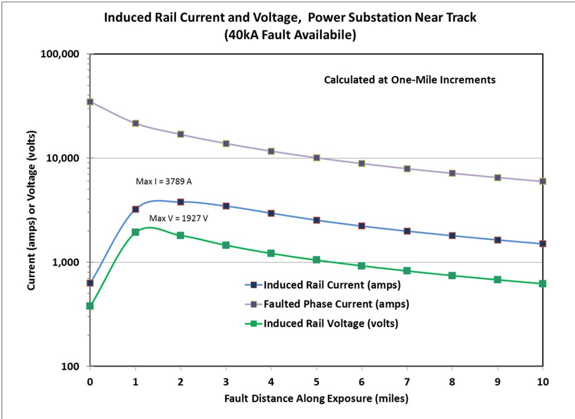
**Figure F-8: Induced Rail Current and Voltage as a Function of the Transmission Line Fault Location**
