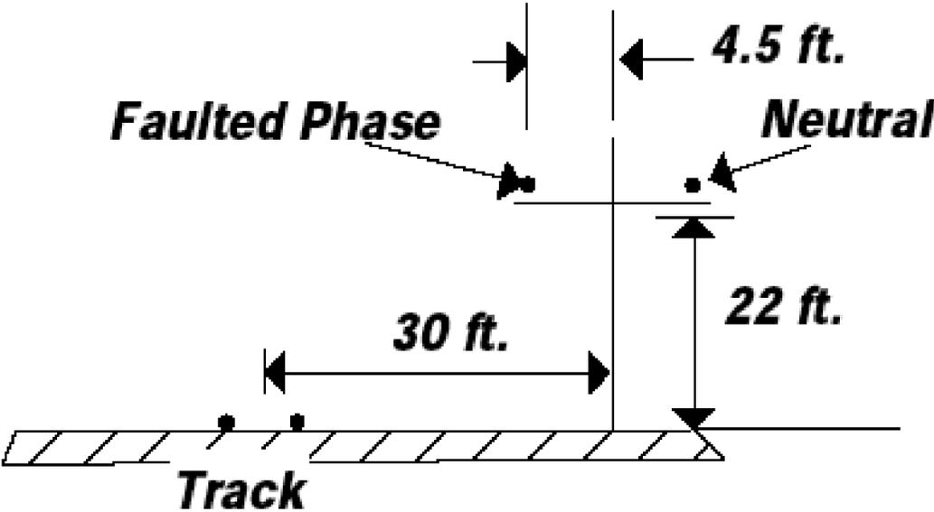
Figure F-4: Cross-Section Distribution Model Geometry
