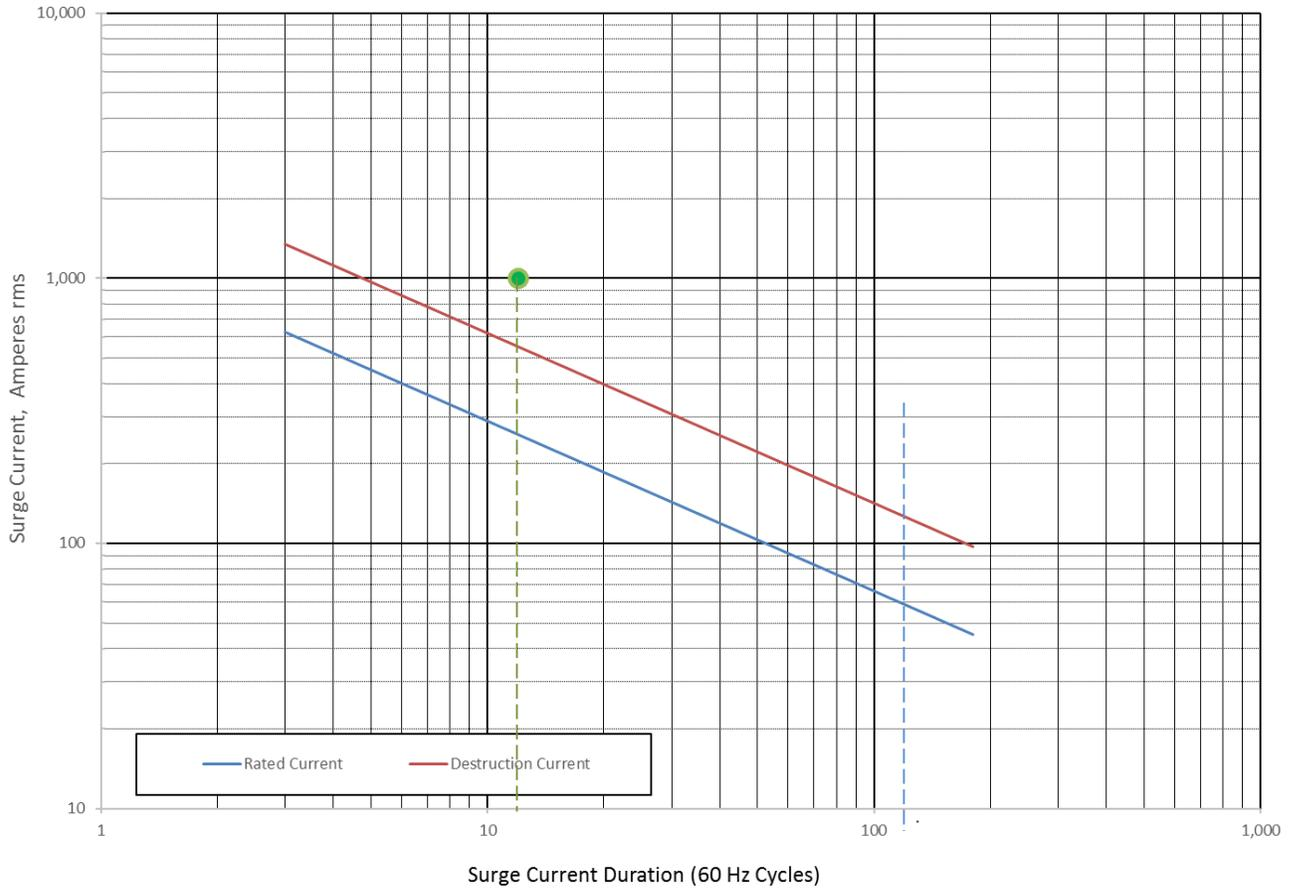
**Figure F-2: Estimated 60 Hz Surge-Current versus Duration in Cycles for Arresters of Figure F-1**
