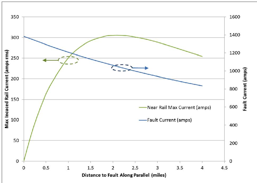
**Figure F-6: Fault Current and Induced Rail Current for Various Fault Locations for a Distribution Line Without a Neutral Wire**
