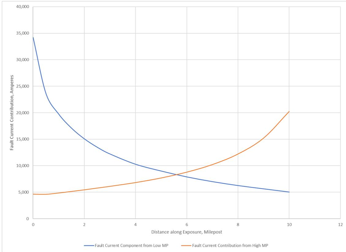
**Figure L-3. Assumed Current Supply from Each Substation to a Fault Along the Parallel Exposure.**
