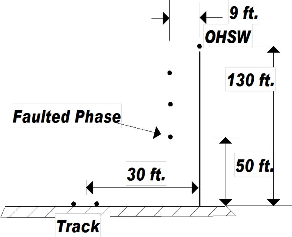
Figure F-7: Cross-Sectional Geometry of Transmission Line
