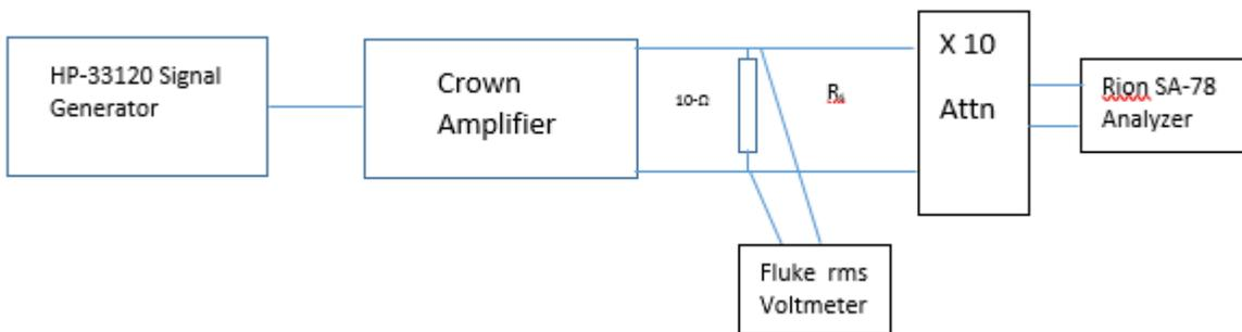
**Figure H-4: Baseline Measurement Circuit Harmonic Measurement Arrangement**
