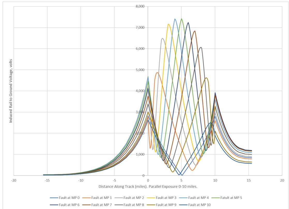
**Figure L-7. Fault-Induced Rail Voltage Curves for Faults at One-mile Increments Along the Parallel Exposure for Assumed Hih Track Ballast Resistivity**
