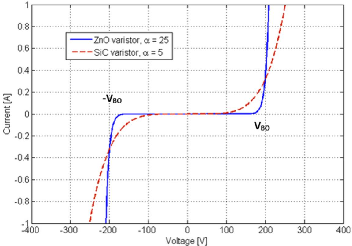
**Figure D-2.: Voltage Current Characteristic of Clamping Device**
