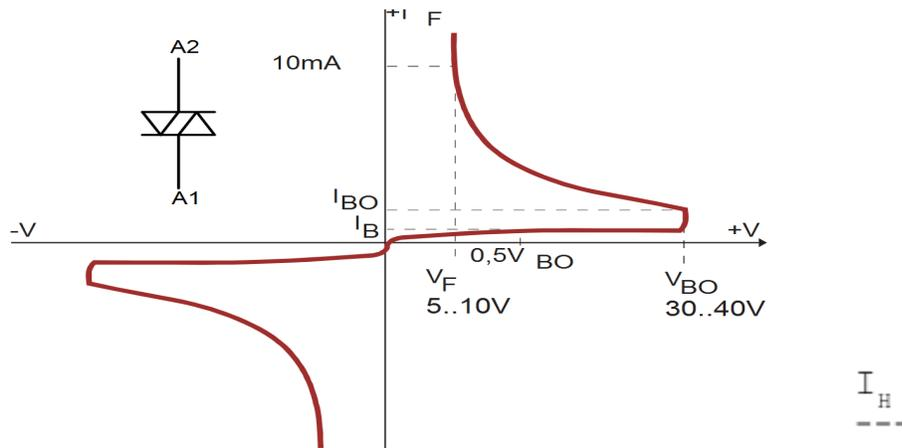
**Figure D-1: Voltage Current Characteristic Representative Of A Crowbar Device.**
