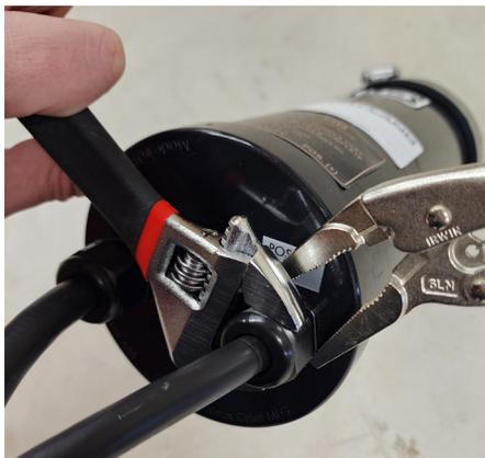
k. Install terminals or splice unfinished ends of wires per application requirements. In any case, take care to seal the ends of the wire so that moisture cannot travel through the wire and into the ENCL-DB enclosure. Refer to SSD or OVP2 literature for guidance on those specific products.
