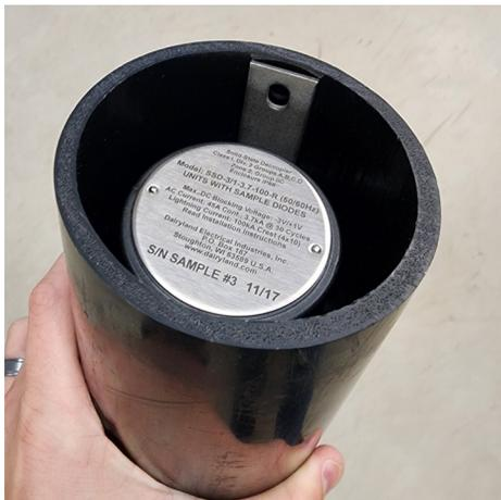
j. Re-install the enclosure cap. Torque clamp screw (size: 5/16" hex) to 60 in-lb.
