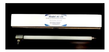
We regret to inform you that we have discovered a dimensional error in the fabrication of the probe tip that will affect the accuracy of the AC-10's readings by 25%. The coupon that you currently have is 8 cm<sup>2</sup>, and not the specified 10 cm<sup>2</sup>.
