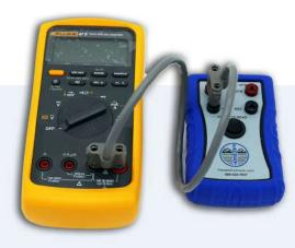
The Ref-Check VPR integrates reliable, medical grade, electronic technology. When used with modern DMMs, it provides a voltmeter sensitivity of over 5 billion ohms input resistance. This exceptionally high input resistance virtually eliminates meter loading to restore an accurate potential reading.
